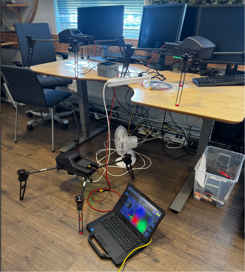
Figure 5.2: Test setup with three Flamingo UAVs and a GCS.
