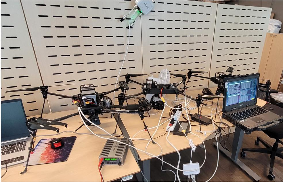
**Figure 6.2:** Ground testing arrangement with three Flamingo drones and one GCS at the laptop to the right
