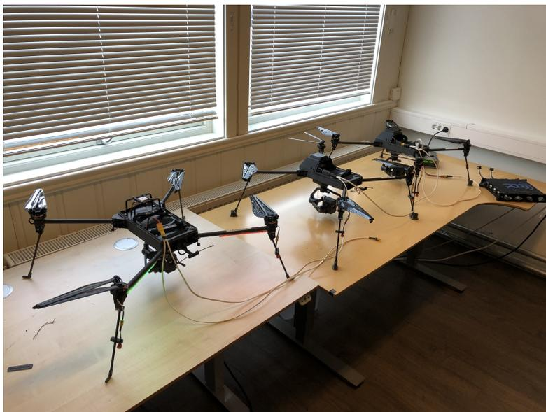
**Figure 5.1:** Physical testbed with three Flamingo drones from the testing conducted at FFI’s location at Kjeller.
