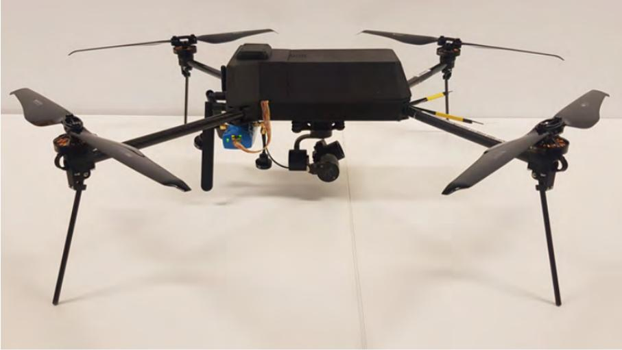
**Figure 2.2:** The Flamingo UAV with a mesh-radio and a thermal camera. The image is retrieved from Nummedal [Num21].
